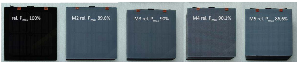
Figure 39: Test modules with white printed glass covers with differing degrees of coverage and print patterns (M2-M5) [65]
