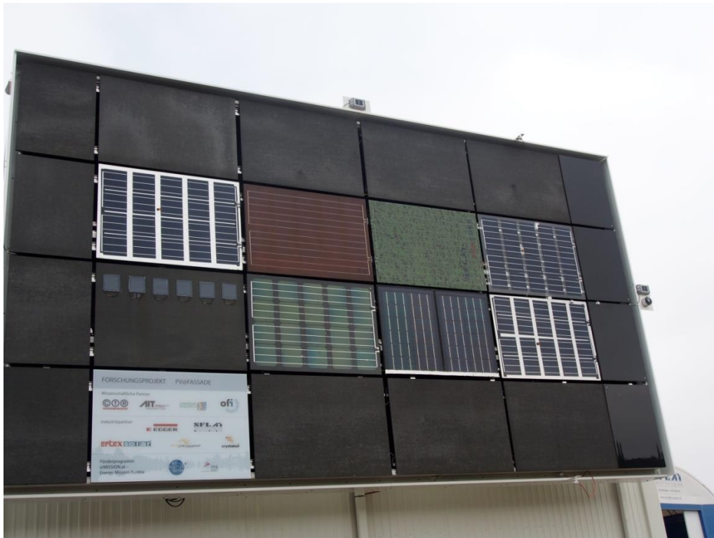
Figure 42: Test façade of innovative BIPV elements developed within project PV@facade with variable back covers, with terracotta coated glass [26], printed glass and coloured Si cells [27];
