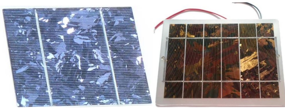
Figure 8: Left: multicrystalline Si solar cell in its original colour; right: multicrystalline Si solar cell with modified thickness of AR COATING (on top of semiconducting material) from Solar Capture Technologies ( www.solarcapturetechnologies.com ).
