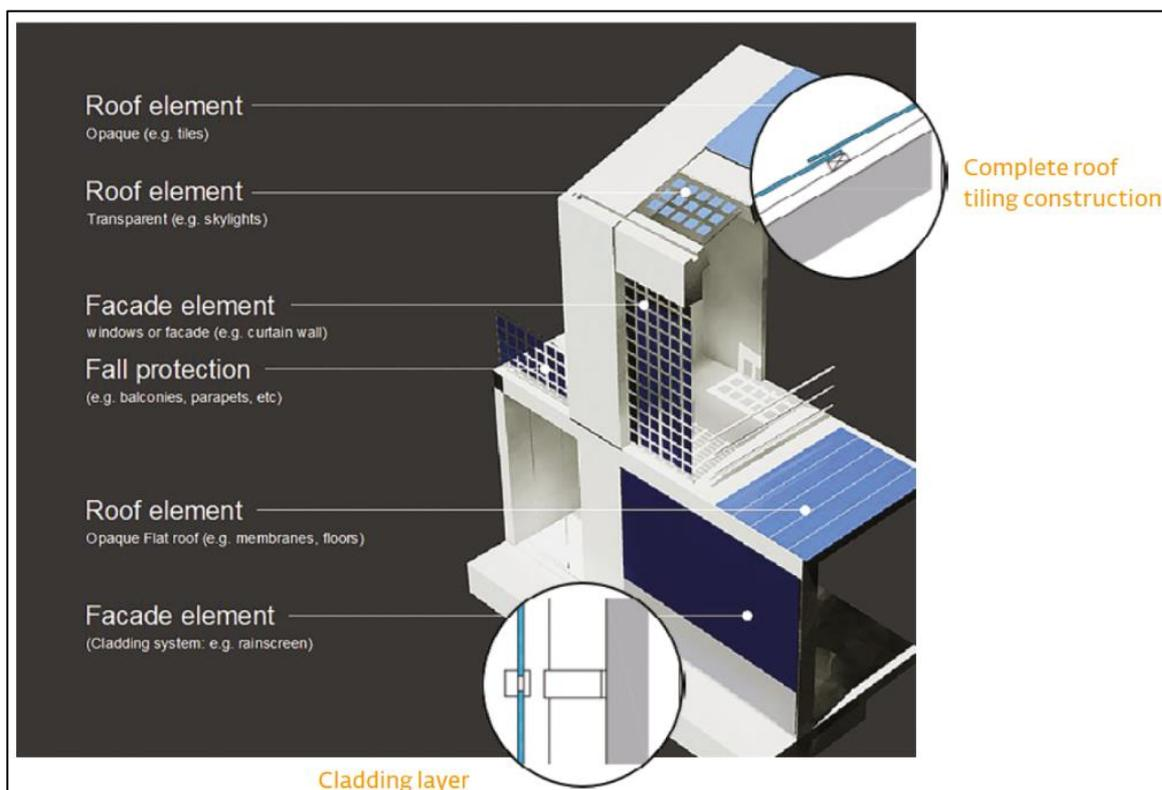
**Figure 3.1** The possible ways to integrate photovoltaic elements into the envelope of a building [1]
