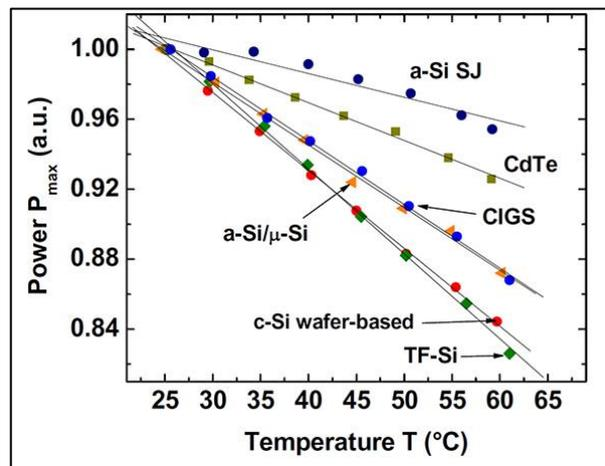
Figure 3.6 Variation of power output with temperature for different solar technologies [25]
